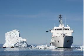
Finnish-built for the Russian Academy of Science, this ship was designed to travel quietly, during hydro-acoustic research. She is exceptionally stable, yet manoeuvrable, with external stabilizers and a built-in trimming system providing exceptional stability. *Akademik Sergey Vavilov* has an ice strengthened hull and a cruising speed in open water of 14.5 knots. She carries a maximum of 94 guests.
